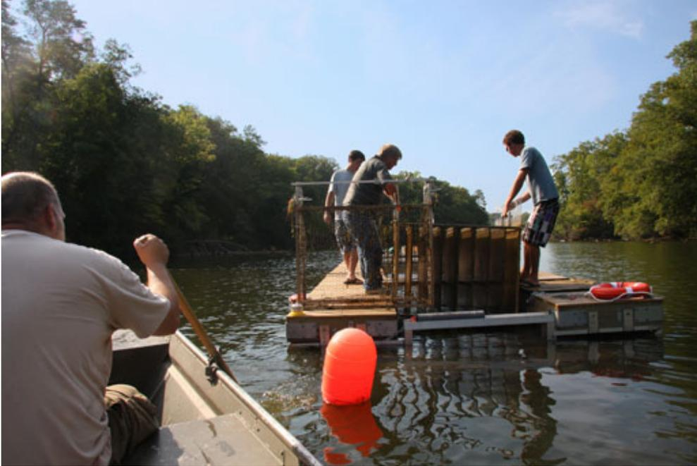
**On the lake:** Karl Kuschner pulls around the Matoaka flume while physicist William Cooke and students work with the substrate screens. The researchers access the Matoaka flume by jonboat, while the York River flume is accessed by a pontoon boat—the R/V Schrödinger’s Cat-amaran—which also serves as a working platform.
